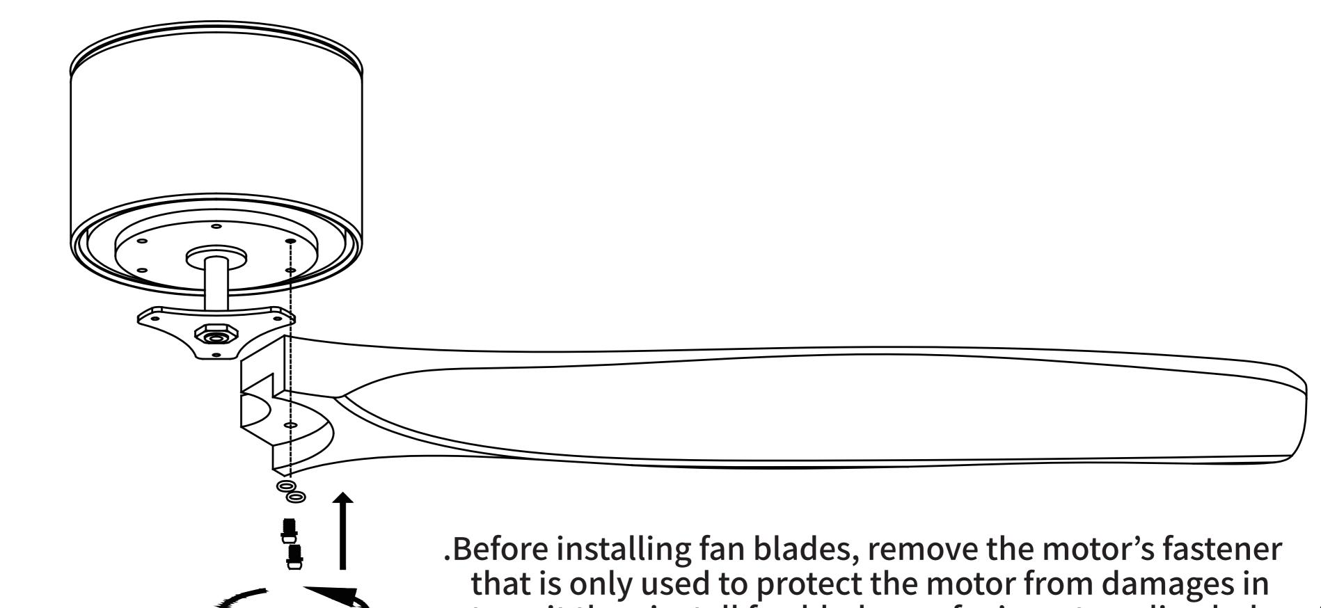
transit then install fan blades on fan's motor, align holes of blades and motor, then screw blades with provided screws. (Figure 6)
