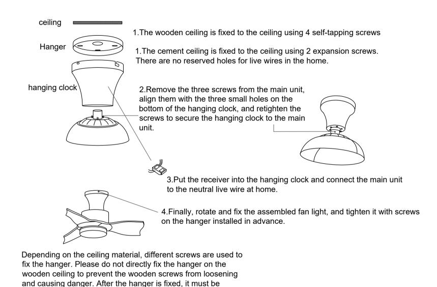
confirmed that it can withstand a gravity of more than 60
