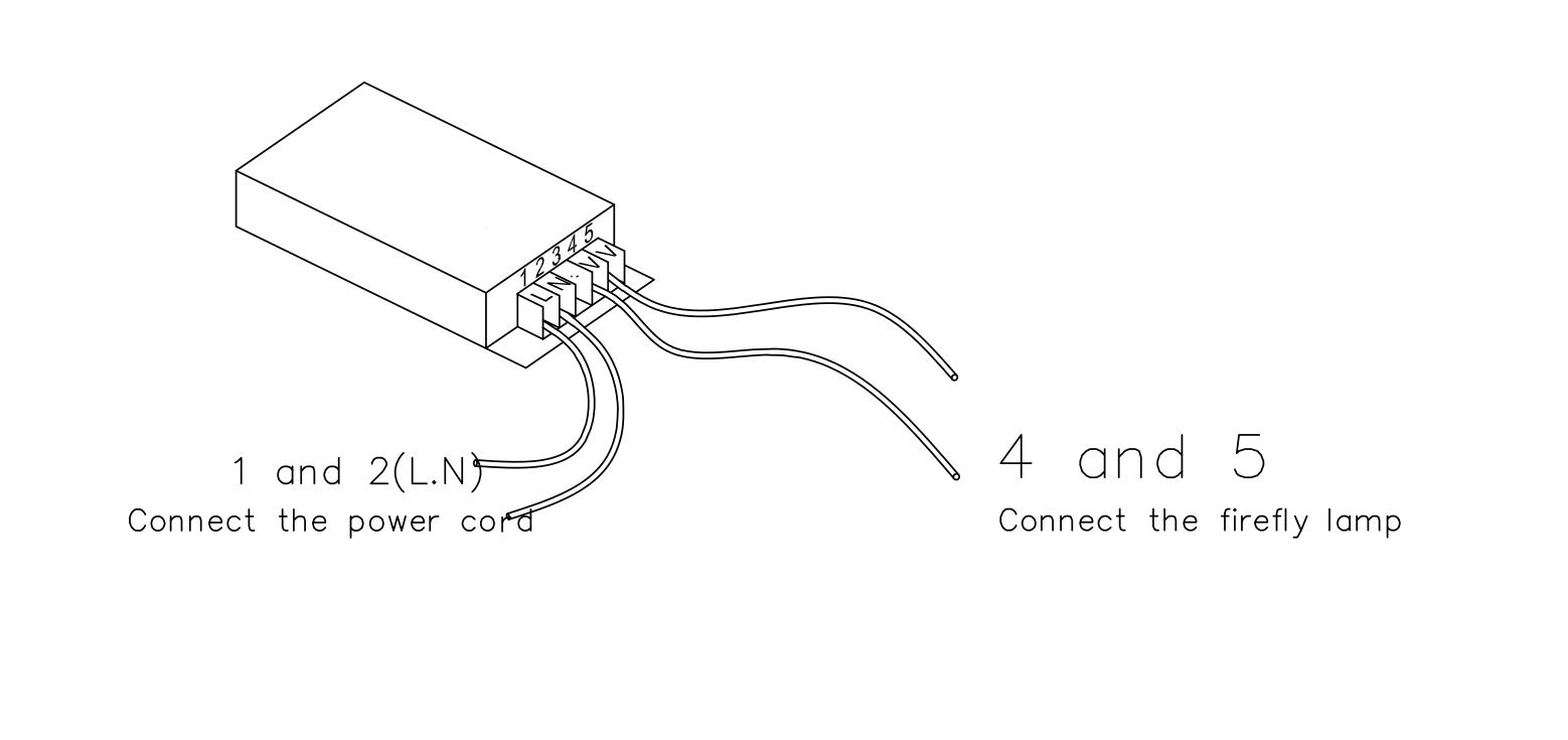
Connect the firefly transformer L and N to the power supply
