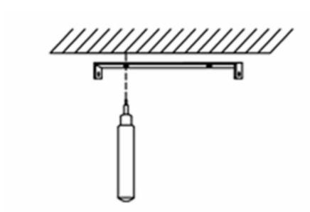
Step1: draw a mark on the ceiling with the hanging board as a reference.
