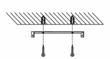
Step4: fix the hanging plate on the expansion screw and tighten it with nuts.
