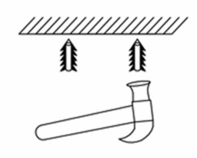
Step3: tap the expansion screw into the drilled hole
