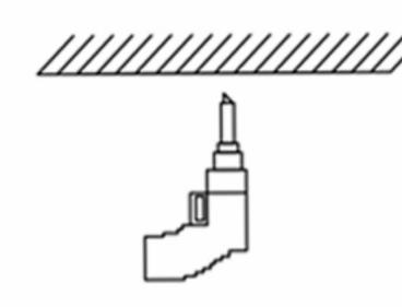
Step2: drill the hanging plate hole on the ceiling with an electric drill.
