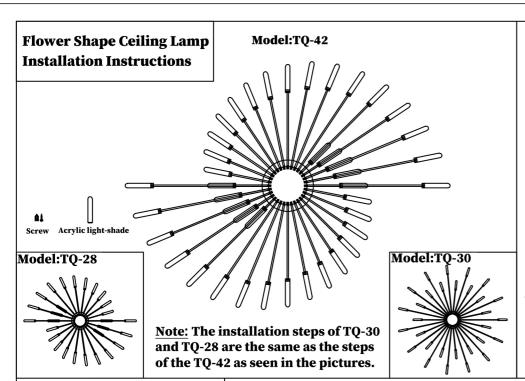
Step1:Open the package and take the ceiling light out. THen Fix each lamp rm tightly into the bace with the nuts as shown in the figure.
